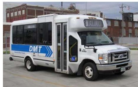
**Figure 4: “Cutaway” Body on Chassis Bus with 24 Seats Used by Danville Mass Transit for Service on Freeway to Champaign**
