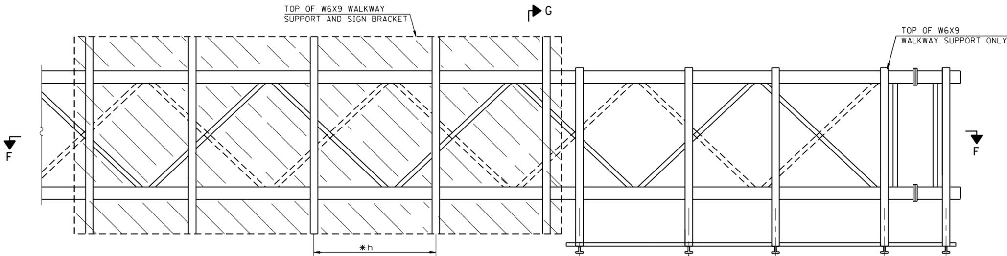
WALKWAY AND TRUSS GRATING WIDTH DIMENSIONS ARE NOMINAL AND MAY VARY ±1/2" BASED ON AVAILABLE STANDARD WIDTHS.
