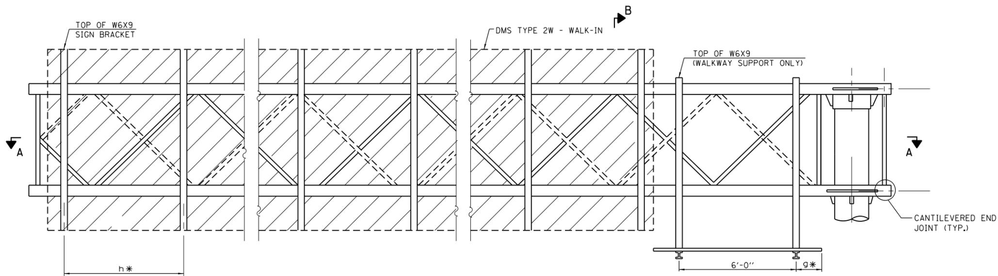
\* BRACKET AND GRATING DIMENSIONS ARE NOMINAL AND WILL VARY BASED ON ACTUAL DMS TYPE 2W - WALK-IN DIMENSIONS PLUS MANUFACTURER'S MOUNTING DEVICES.
