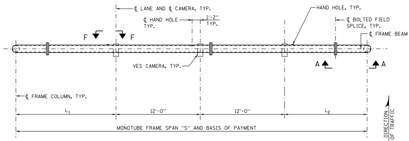
**AET RAMP EXIT MONOTUBE PLAN**
