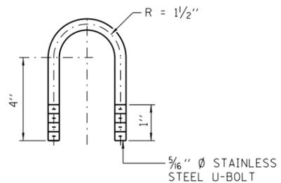
DAMPING DEVICE MOUNTING TUBE U-BOLT DETAIL (TYPICAL)
