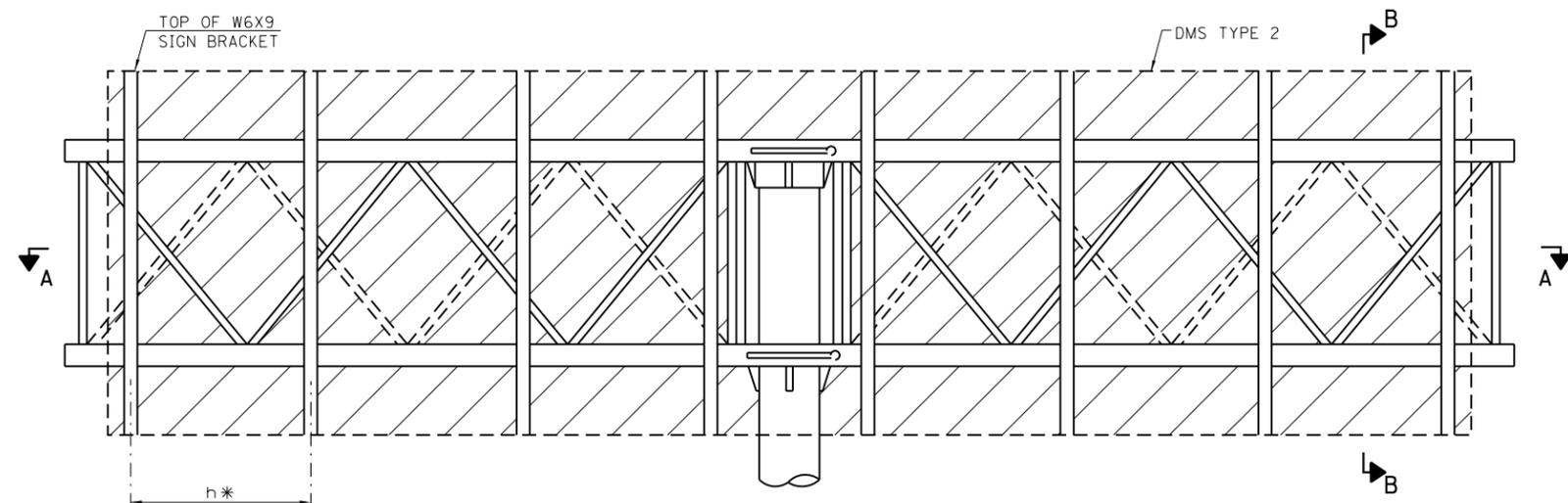
\* BRACKET DIMENSIONS ARE NOMINAL AND WILL VARY BASED ON ACTUAL DMS TYPE 2 DIMENSIONS PLUS MANUFACTURER'S MOUNTING DEVICES.
