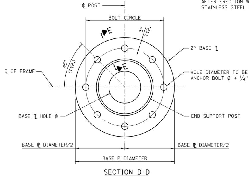
FOR UT, GRIND TOP OF BOLT SQUARE AND SMOOTH BEFORE GALVANIZING.
