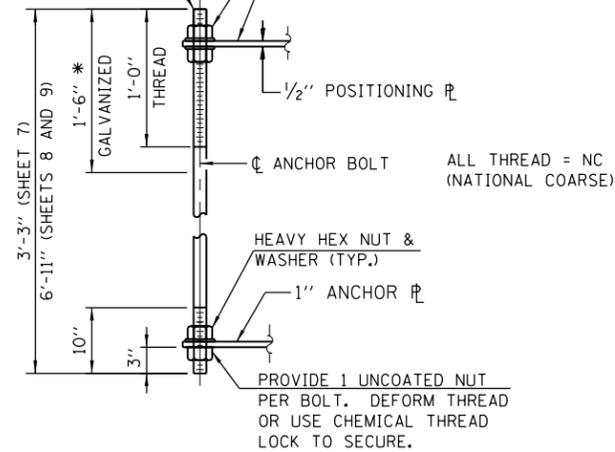
ANCHOR BOLTS SHALL CONFORM TO AASHTO M314 GRADE 105 AND MEET CHARPY V-NOTCH (CVN) ENERGY OF 15 LB.-FT. AT 40° F. GALVANIZE UPPER 18" PER AASHTO M232. NO WELDING SHALL BE PERMITTED ON BOLTS.
