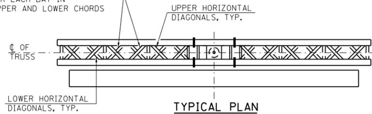
ALTERNATE VERTICAL DIAGONAL BRACING FOR EACH BAY IN PLANES OF FRONT AND BACK CHORDS
