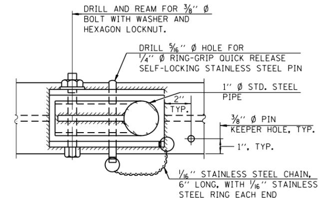
**PLAN AT HANDRAIL HINGE**
