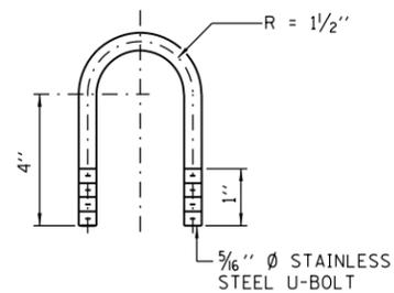
DAMPING DEVICE MOUNTING TUBE U-BOLT DETAIL (TYPICAL)
