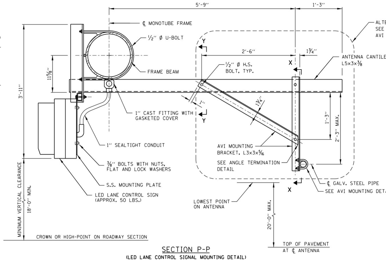
**SECTION P-P (LED LANE CONTROL SIGNAL MOUNTING DETAIL)**
