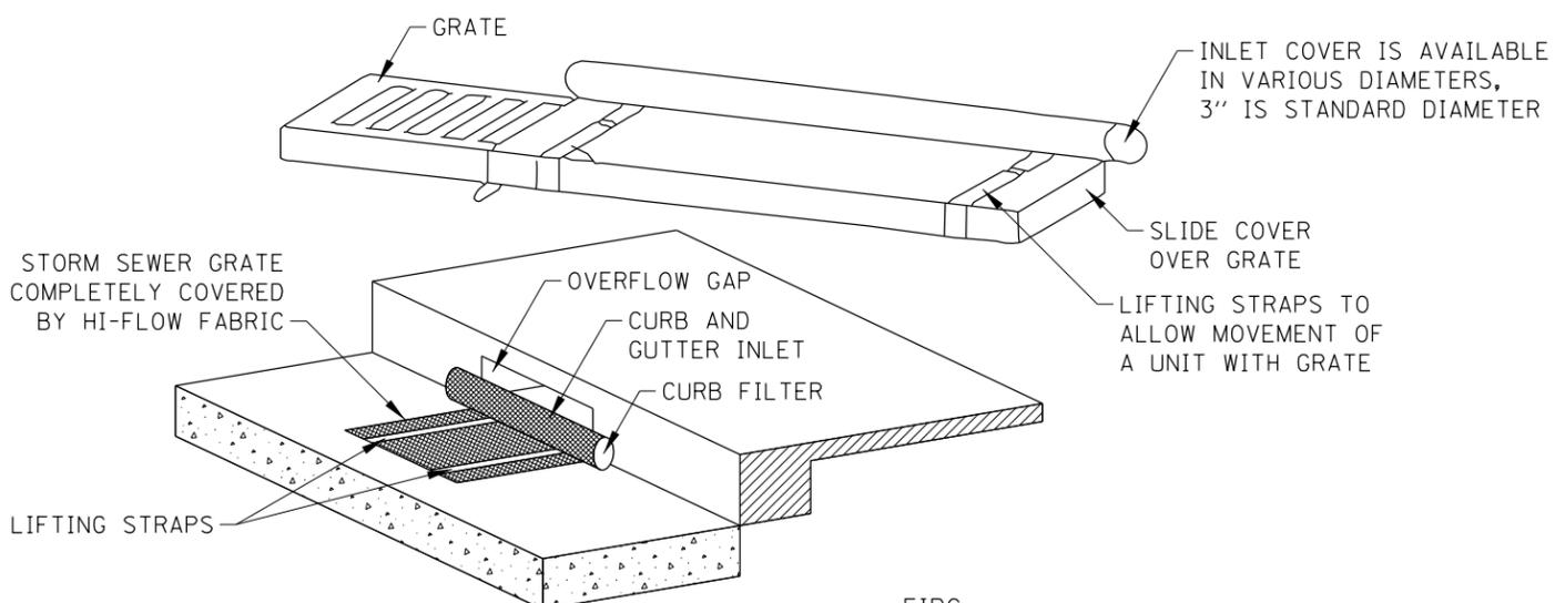
STORM SEWER GRATE COMPLETELY COVERED BY HI-FLOW FABRIC
