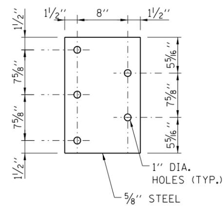
PARAPET STEEL BEARING PLATE DETAIL
