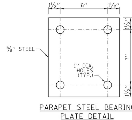
(4 EACH INDIVIDUAL 5"x5"x5/8" STEEL PLATES WITH CENTERED HOLES MAY BE SUBSTITUTED FOR THE PLATE SHOWN)
