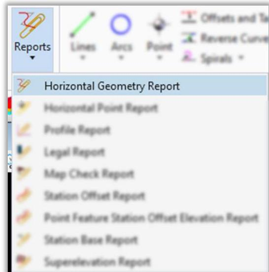
Select the desired 2-D corridor feature to be analyzed and follow the *Horizontal Geometry Report* tool prompts. For this example, select the corridor feature with the *Complex Element: EOP\_HMA 12* (edge of right lane).
