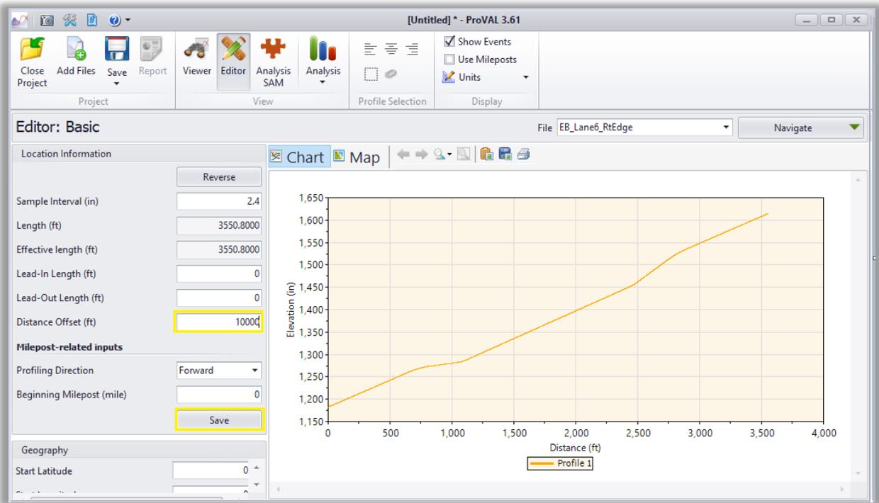
The distance along the X-axis will be adjusted to reflect the starting station of the project.
