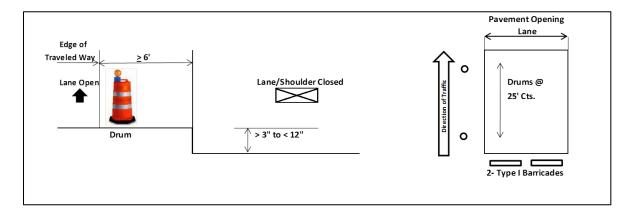
Additional drums are to be placed at 25-foot centers adjacent to the drop-off area for a minimum of 100 feet or the length of the drop-off area, whichever is greater.
