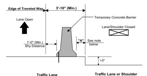
When dimension "A" is less than 3'- 6" the temporary concrete barrier shall be anchored to pavement or deck. Anchor pins shall not be installed through bridge decks, on bridge approach slabs and continuously reinforced concrete tolling zone pavements that are new or existing to remain in place. Anchor pins should not be installed through transition approach slabs that are new or existing to remain in place. Reference Article 6.4.7 of this MOT MANUAL for barrier anchorage systems.
