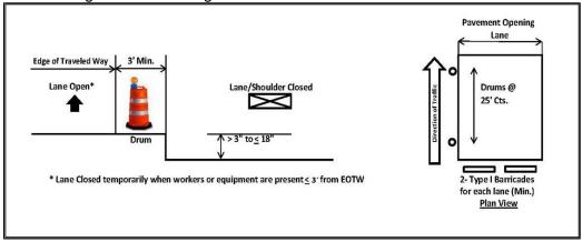
For each pavement opening, Type I barricades shall be placed in front of the opening. A minimum of two (2) Type I barricades shall be installed for each lane. The barricades shall remain for a period beginning immediately after removal is completed and until the curing period for the new concrete pavement has elapsed and all debris has been cleared away or until the excavated depth is less than 3 inches.
