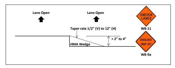
Drop-offs of  $\leq$  3 inches adjacent to traffic carrying lanes are permitted without tapers or TCB. The minimum distance from edge of traveled way to edge of drop-off is 3 feet. Spacing of traffic control devices shall be in accordance with the applicable Illinois Tollway Standard Drawing.
