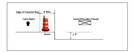
Drop-offs of > 3 inch to < 18 inches adjacent to traffic carrying lanes are permitted without tapers or temporary concrete barriers provided a distance of 3 feet from the edge of traveled way to edge of drop-off is available for the placement of traffic drums or barricades. Spacing of traffic control devices shall be in accordance with the applicable Illinois Tollway Standard Drawing.
