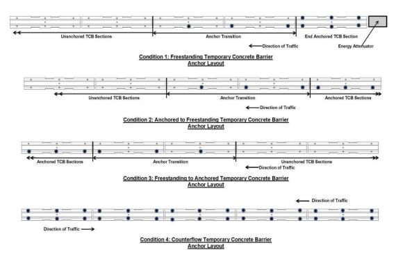
Figure 3 – Temporary Concrete Barrier Layouts
