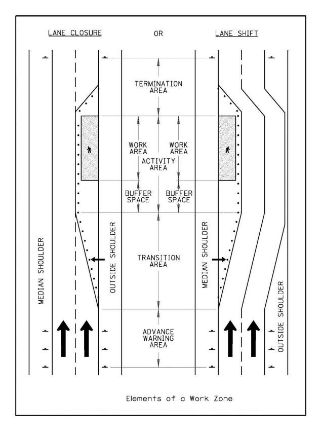
Figure 2 – Element of a Work Zone
