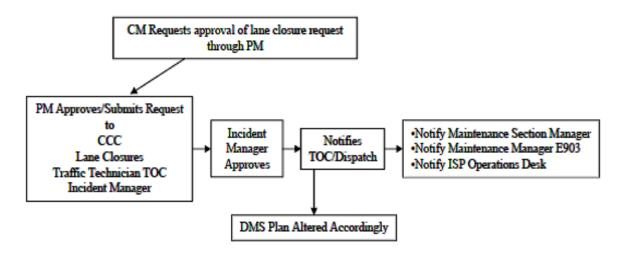
Figure 1 - Emergency Lane Closure Request/or After Hour Lane Closure Changes
