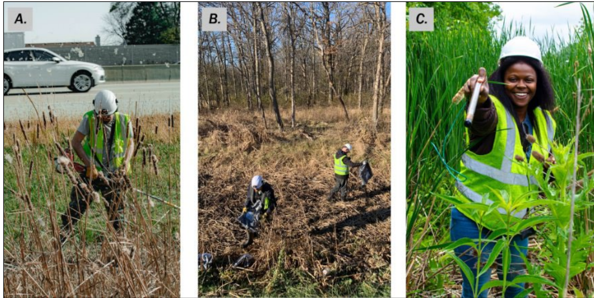
Figure 3 A. Harvest plot establishment (Oct 2022), B. Biochar application [20 T/ha (17,843 lb/acre)] (Oct 2022), C. Probe Installation and Monitoring (Dec 2022 – November 2024).
