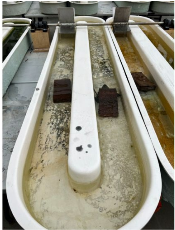
Figure 17 Sodium chloride and fertilizer were added at respective treatment rates: Salt (0.0 mg/L, 500 mg/L), phosphorus (0 mg/L, 0.1 mg/L, 3.5 mg/L), and nitrogen (0 mg/L, 2.0 mg/L, 20 mg/L). For five weeks, individual wood-waste biochar bags were removed weekly for chemical analysis.
