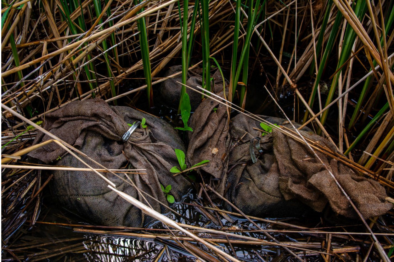
Figure 4 Original jute biochar sacks deployed at the end of each bioswale block to investigate biochar chemical surface adsorption and biochar saturation rates. These biochar bags were replaced with plastic flow-through bags which were sampled at five-time intervals to establish the biochar saturation curve in the field.
