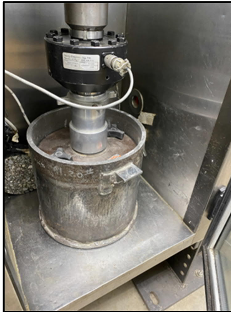
FIGURE 20. Axial compression compaction by closed-loop servo-hydraulic test machine
