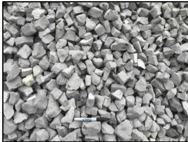
FIGURE 2. Foamed glass aggregate manufactured (Loux et al., 2019).
