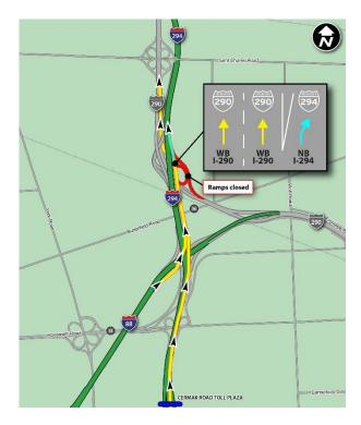
Once the new fly-under ramp is open, northbound I-294 traffic traveling to westbound I-290 will exit the mainline onto auxiliary lanes on the right and then will be directed to use the two left lanes to access the new fly-under ramp which will now provide two lanes traveling under the I-294 mainline to access westbound I-290. Drivers in the right lane will continue on to I-294 northbound.
