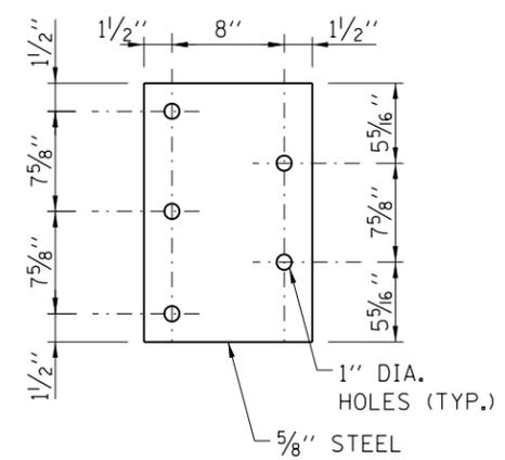
PARAPET STEEL BEARING PLATE DETAIL
