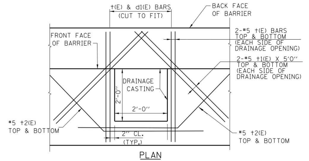
**REINFORCEMENT AROUND DRAINAGE STRUCTURE**
