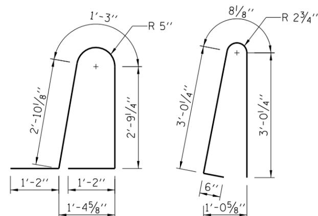
BAR d1(E) BAR d(E) BENDING DIAGRAMS
