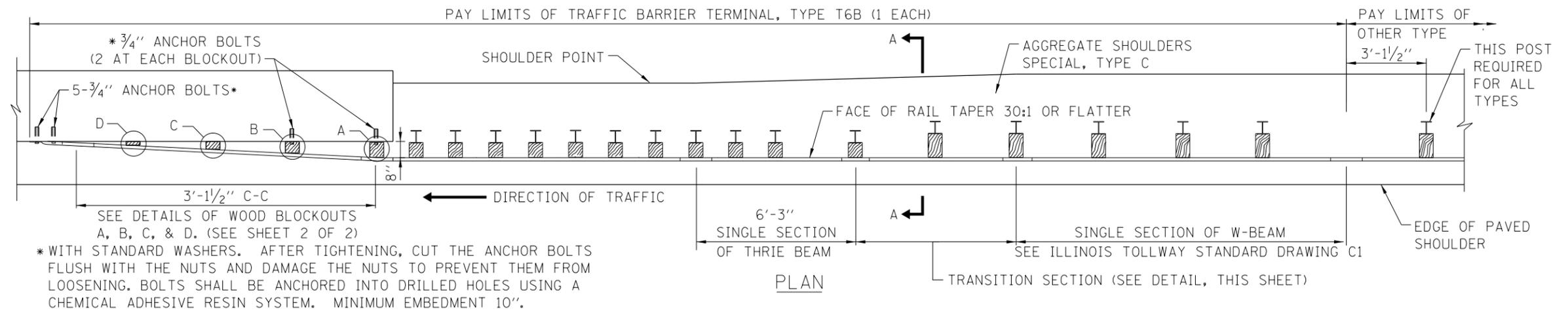
\* WITH STANDARD WASHERS. AFTER TIGHTENING, CUT THE ANCHOR BOLTS FLUSH WITH THE NUTS AND DAMAGE THE NUTS TO PREVENT THEM FROM LOOSENING. BOLTS SHALL BE ANCHORED INTO DRILLED HOLES USING A CHEMICAL ADHESIVE RESIN SYSTEM. MINIMUM EMBEDMENT 10".
