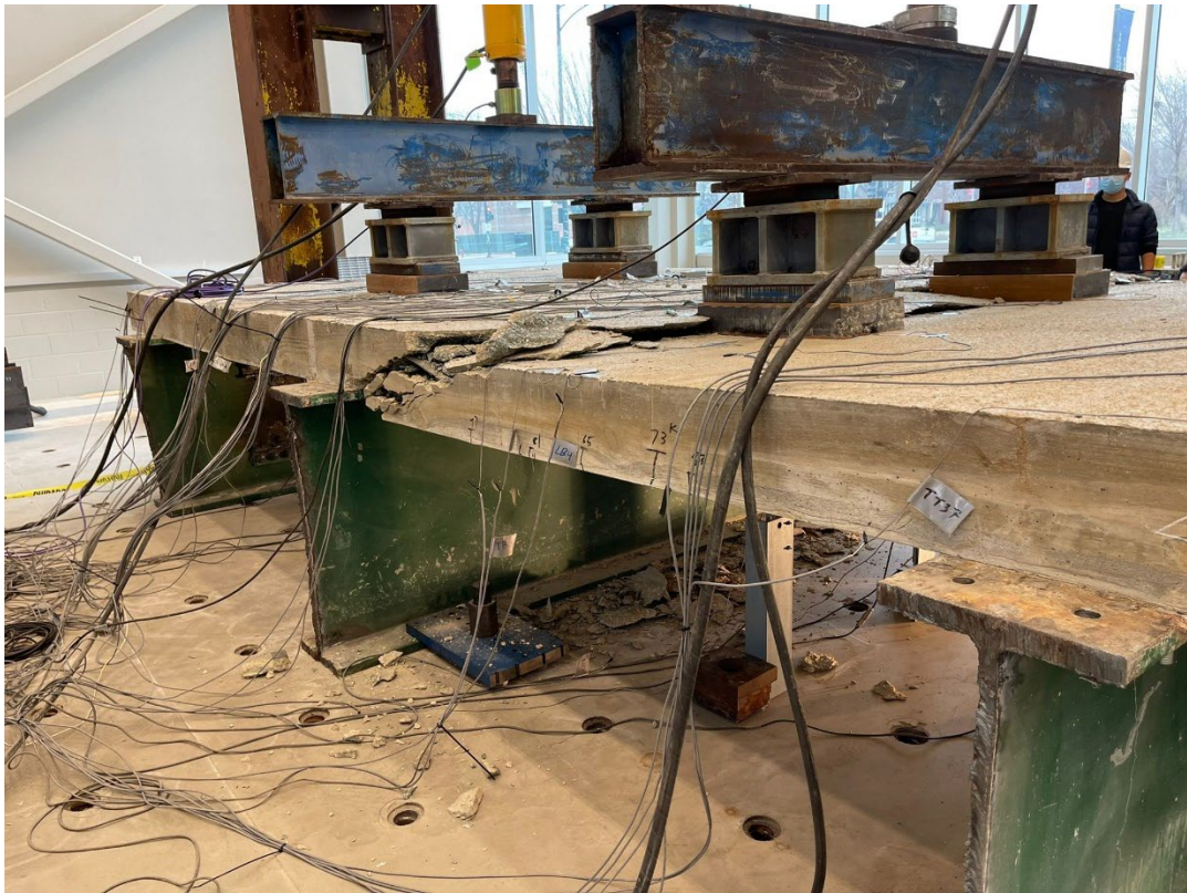
Figure 106: Failure mode of the two-span Prototype 5.
