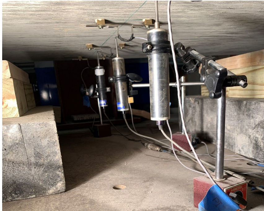
Figure 49: LVDTs and the Pi-shape Displacement Transducers at the bottom midspan of the deck
