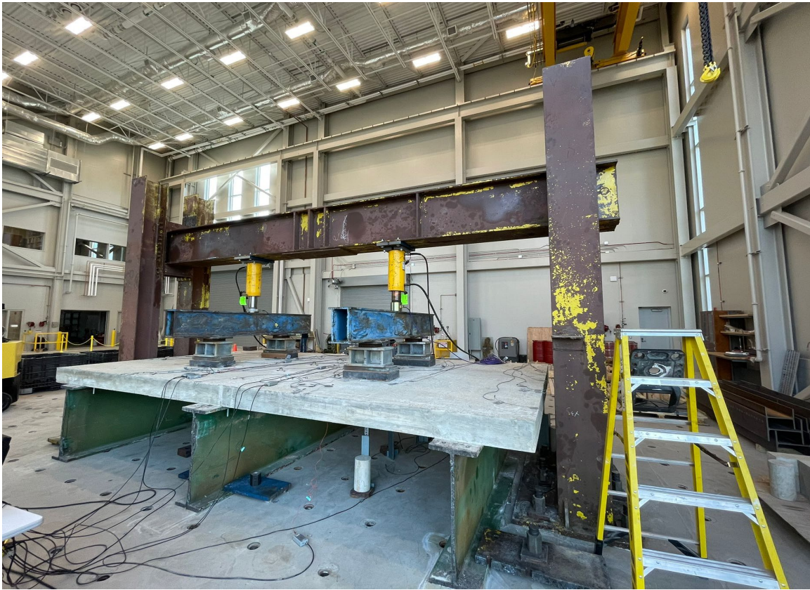
Figure 104: Testing setup of two-span continuous bridge deck slab Prototype 5.
