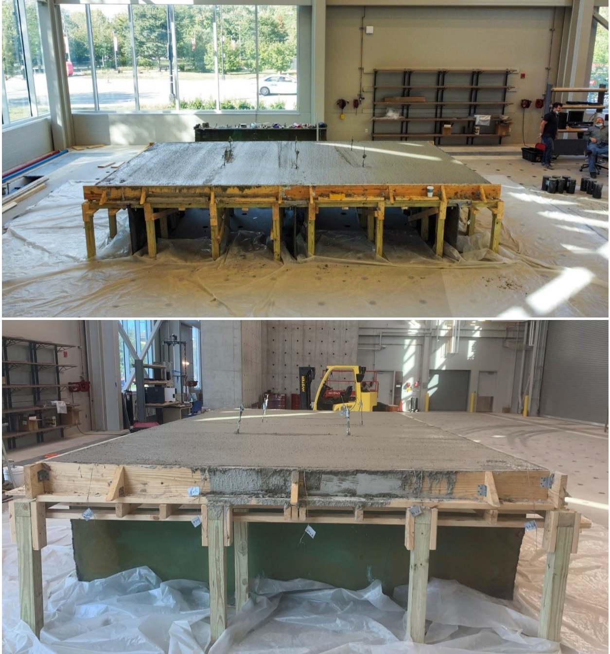
Figure 96: Continuous bridge deck Prototype 5 during and after concrete pouring.
