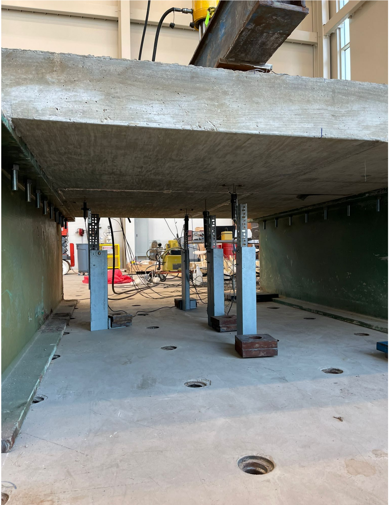
Figure 105: Instrumentation at the bottom concrete surface of the two-span Prototype 5.
