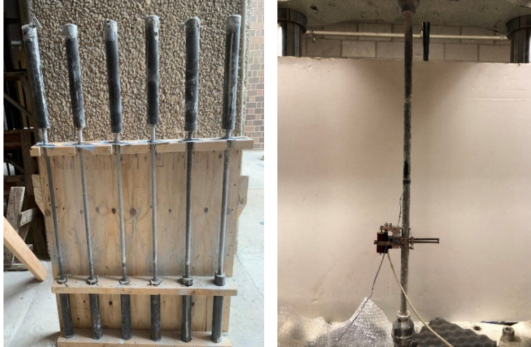
Figure 6: Tensile test sample preparation and test setup.
