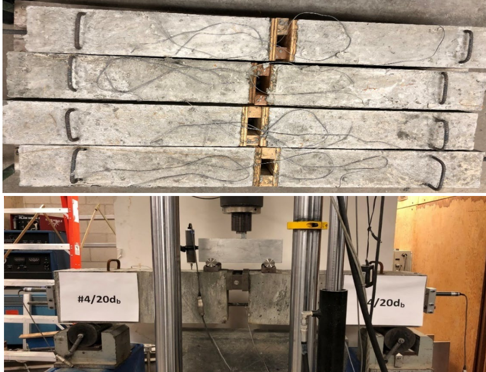
Figure 15: Hinged beam and test setup.
