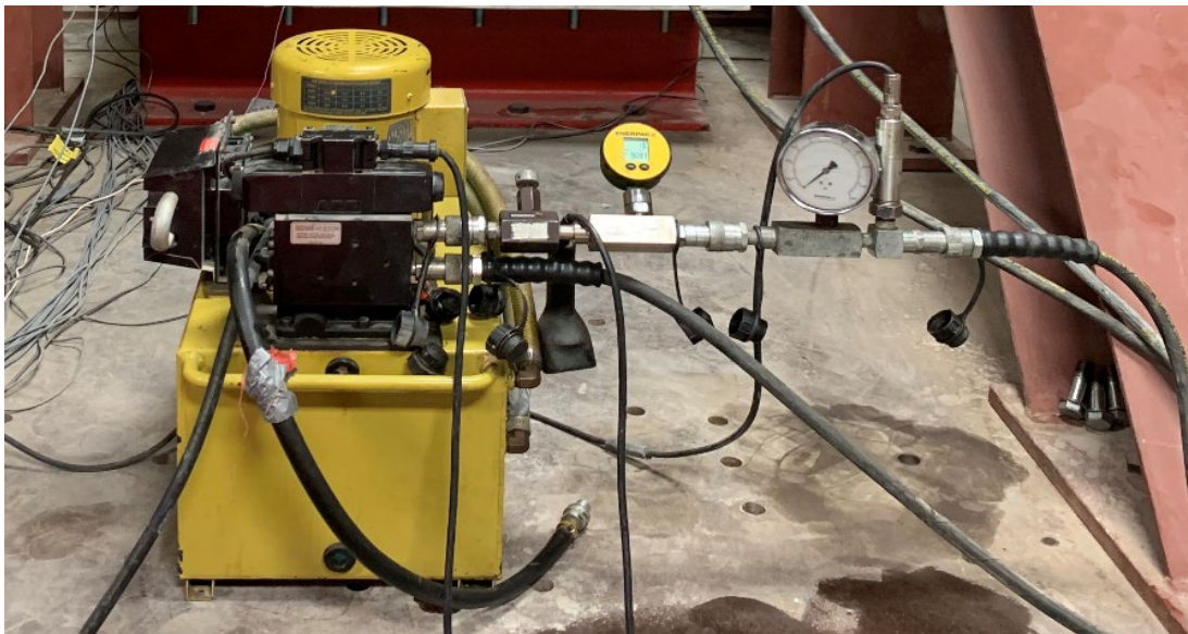
Figure 52: Pressure gauges attached to the hydraulic pump
