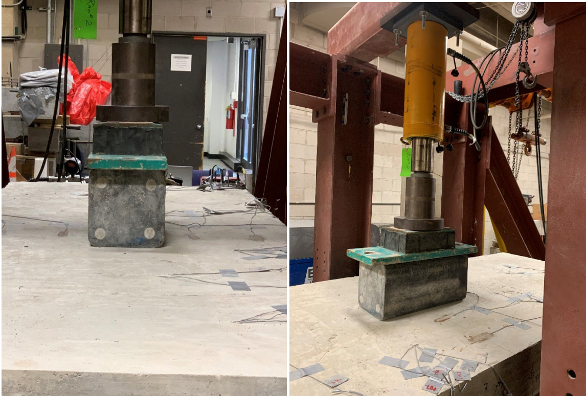
Figure 53: HDPE recycled plastic material fixture simulating wheel contact area of 20 in.x10 in.
