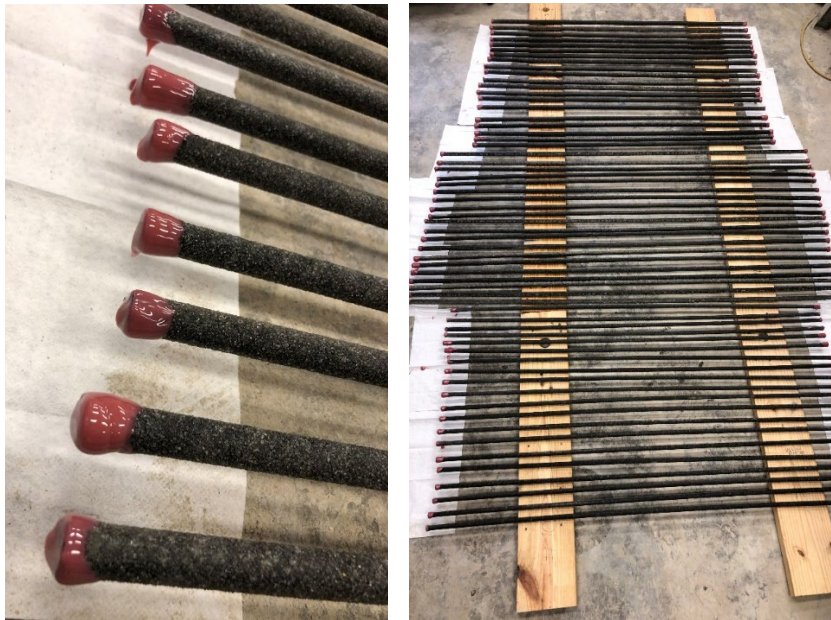
Figure 33: Alkaline test samples preparation.
