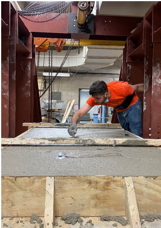
Figure 48: Cast of the first single-span bridge deck slab
