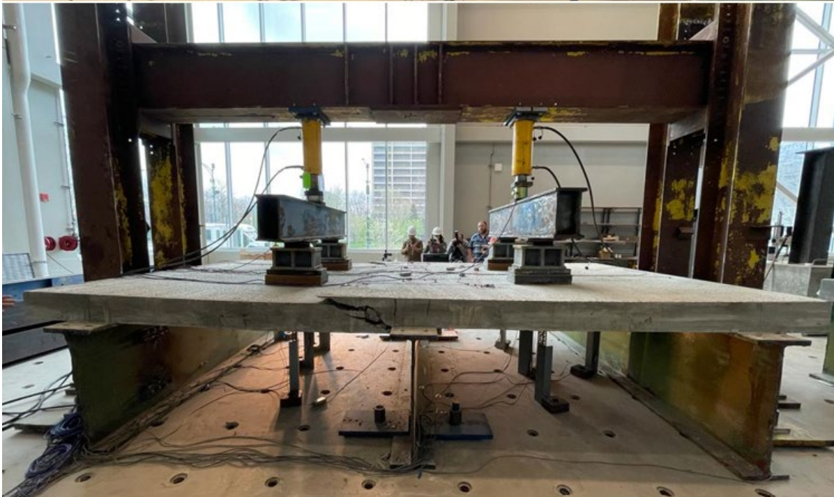
Figure 125: Typical mode of failure of two-span bridge deck Prototypes.
