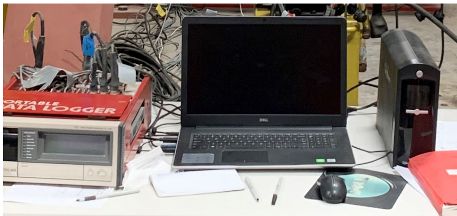
Figure 50: Data acquisition system connected to the laptop
