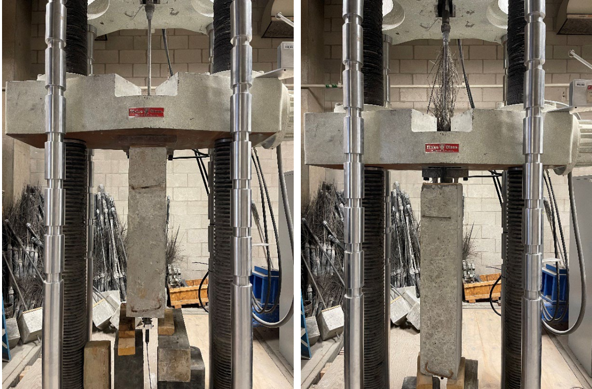
Figure 24: Pullout testing setup of 40db and 50db.
