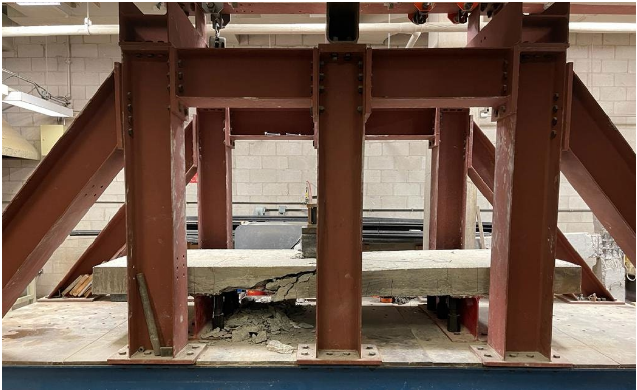
Figure 80: Mode of failure of bridge deck Prototype 3.
