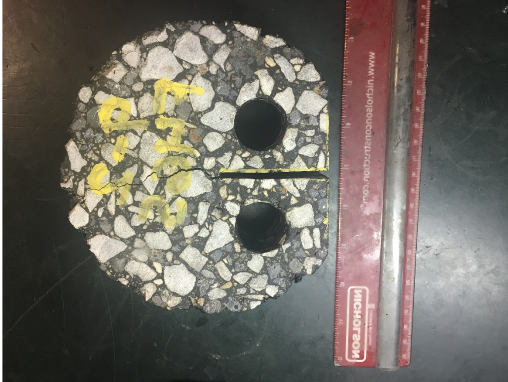
Figure 4. Fabricated DC(T) specimen from the plant-compact gyratory sample
