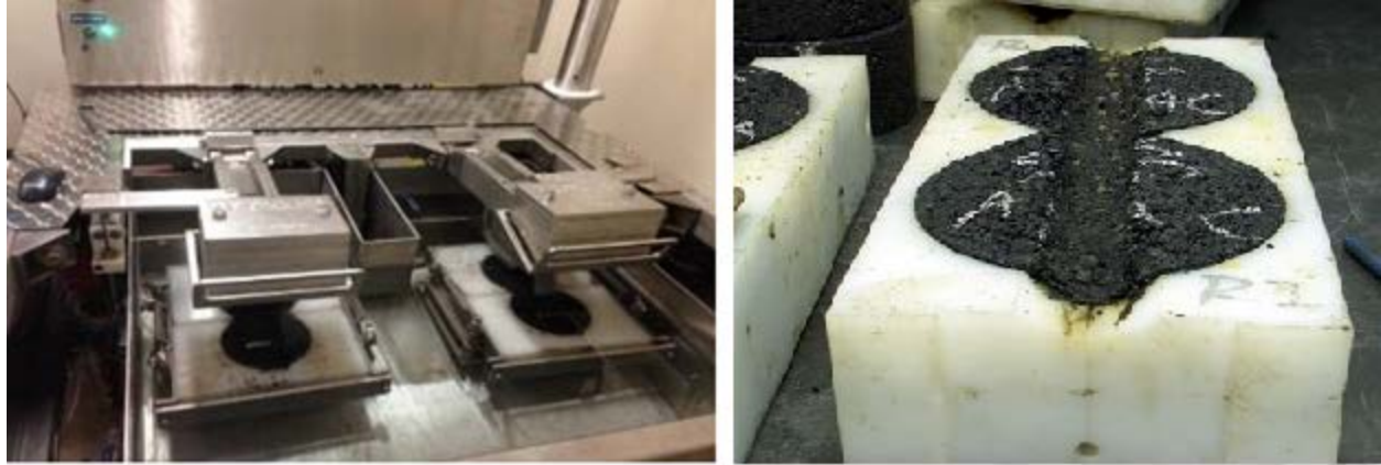
Figure 5. Hamburg Wheel Tracking Device: a) During test b) After test
