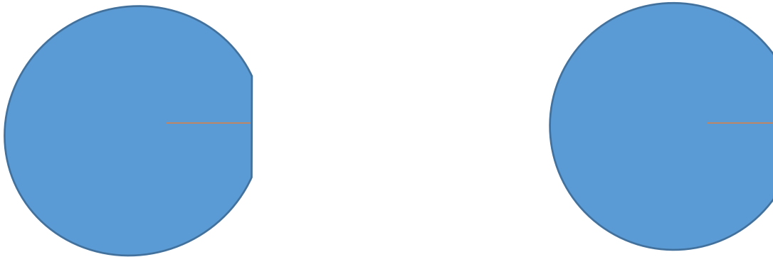
Figure 28. DC(T) specimens, a) standard specimen with notch length = b, b) non-standard specimen with notch length = b 1
