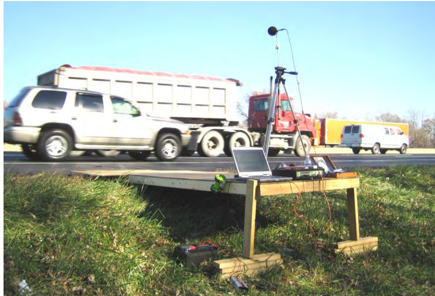
Figure 1. microphone and laptop computer set up on the plywood platform.
