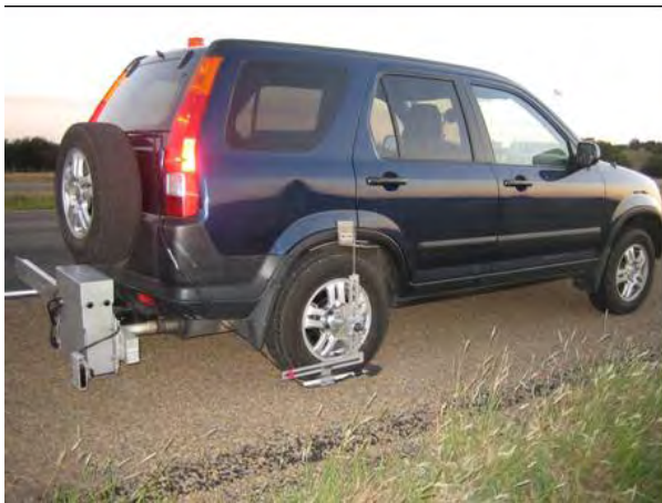
Figures 1 and 2 show the sound intensity microphones mounted to the test vehicle.
