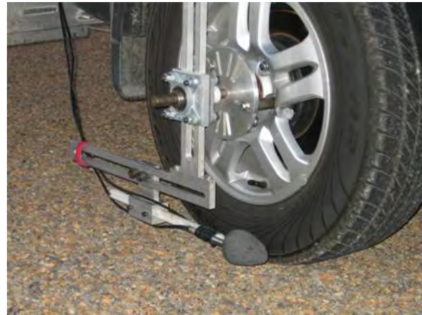
Figures 1 and 2 show the sound intensity microphones mounted to the test vehicle.
