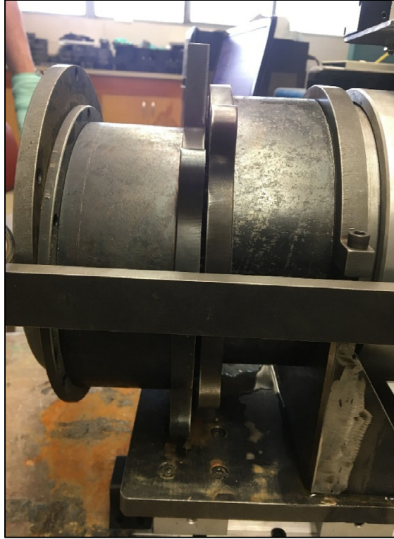
FIGURE 44. Direct shear test set-up.
