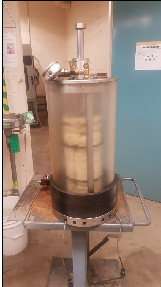
FIGURE 49. Triaxial test set-up.
