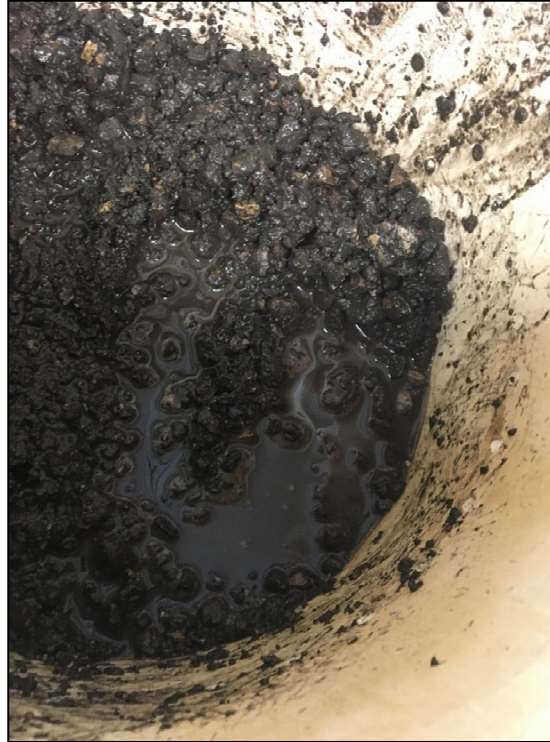
FIGURE 61. Water stored in RAP layer after PGE removal.
