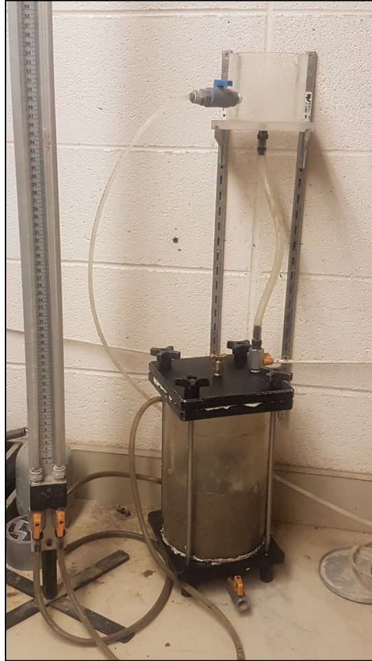
FIGURE 46. Constant head/falling head permeability test equipment.
