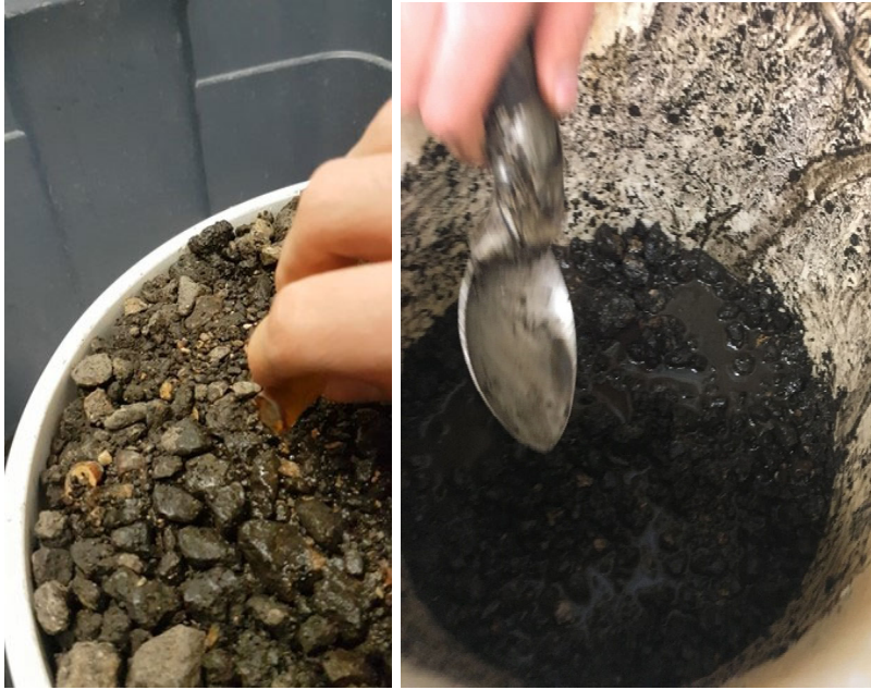
FIGURE 63. Introduction of water to RAP directly (left) and water in RAP during removal (right).
