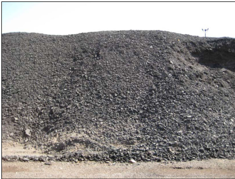
FIGURE 1. Unprocessed RAP from a single stockpile (Copeland, 2011).
