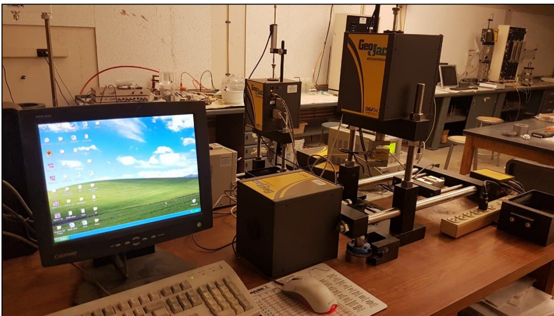
FIGURE 42. First test set-up (GeoJac) for one-dimensional consolidation testing.
