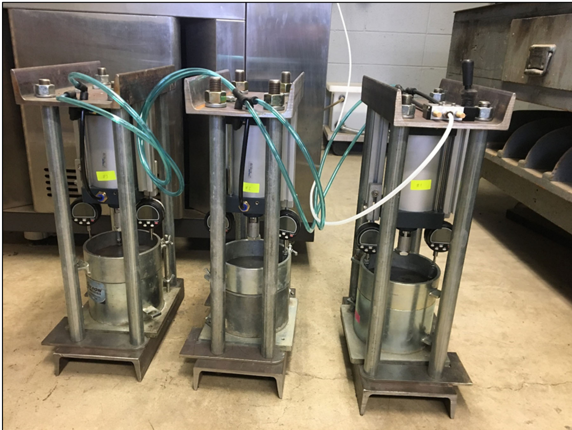
FIGURE 43. Second test set-up (equipment fabricated at WSU) for one-dimensional consolidation testing.
