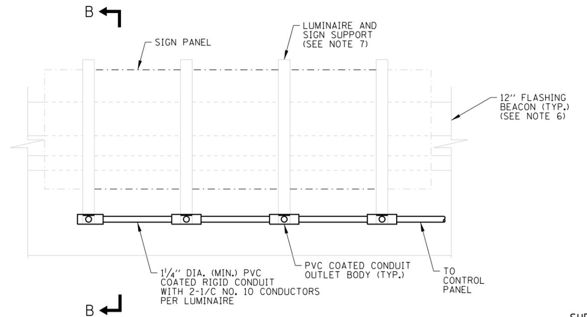
**TYPICAL FRONT ELEVATION WITHOUT FLASHING BEACON**
