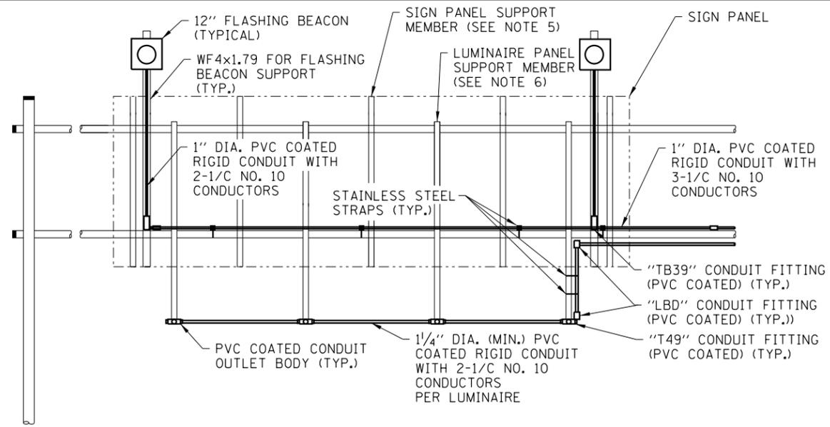
**FRONT ELEVATION WITH FLASHING BEACON**
