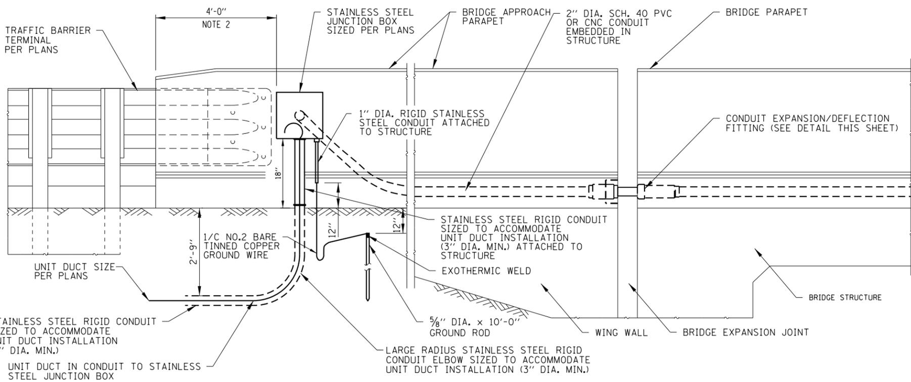
**CONDUIT EMBEDDED IN BRIDGE PARAPET WALLS
