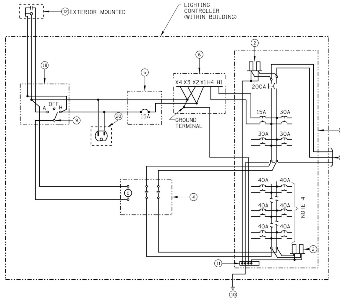
CONTROL CONSOLE WIRING DIAGRAM
