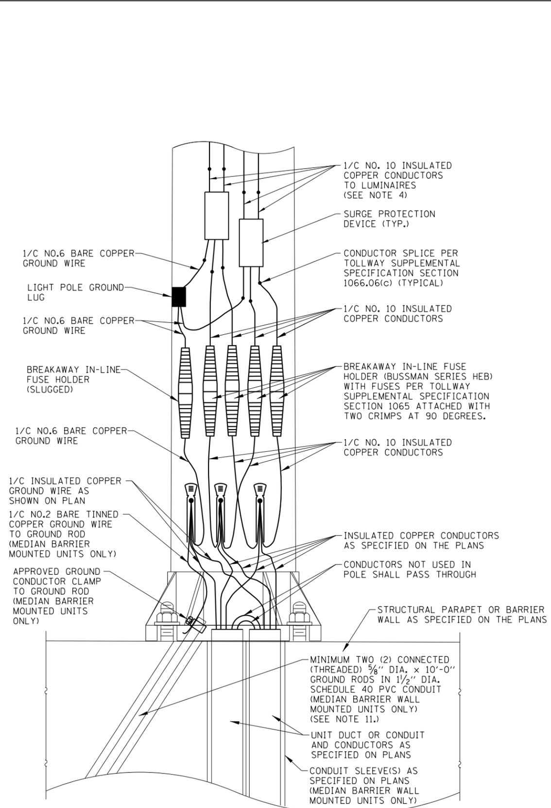
**LIGHT STANDARD WIRING DETAIL**
