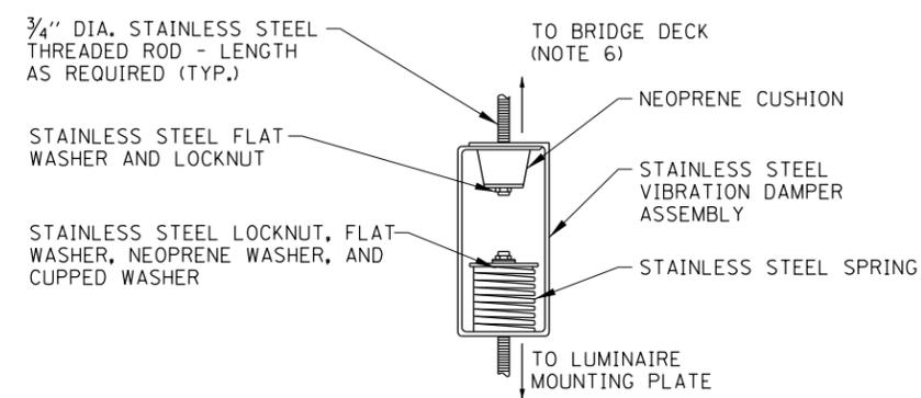
LUMINAIRE HANGER ASSEMBLY DETAIL
