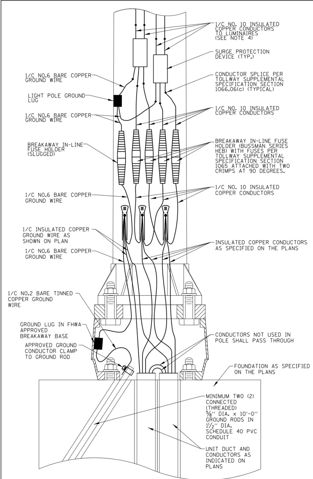
**LIGHT STANDARD WIRING DETAIL**
