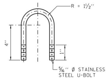
DAMPING DEVICE MOUNTING TUBE U-BOLT DETAIL (TYPICAL)
