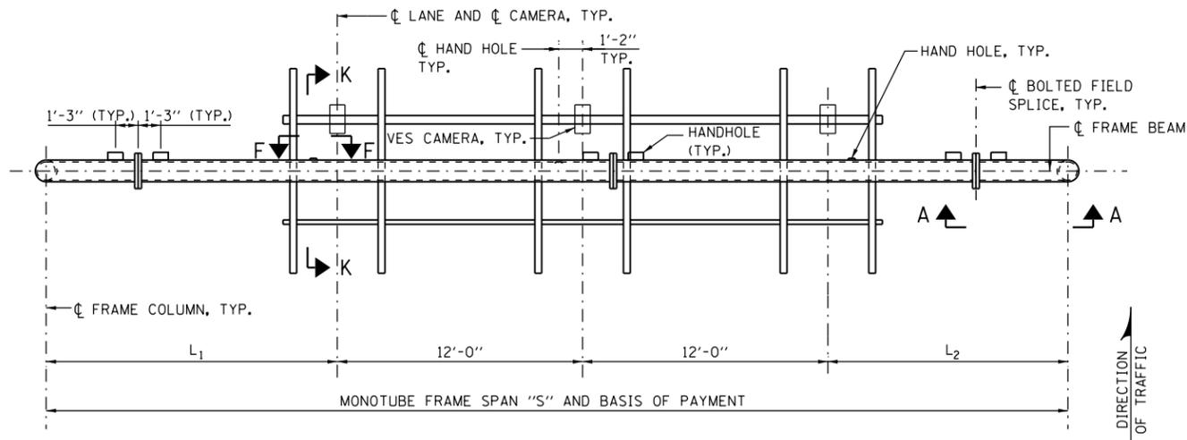
**AET RAMP EXIT MONOTUBE PLAN**
