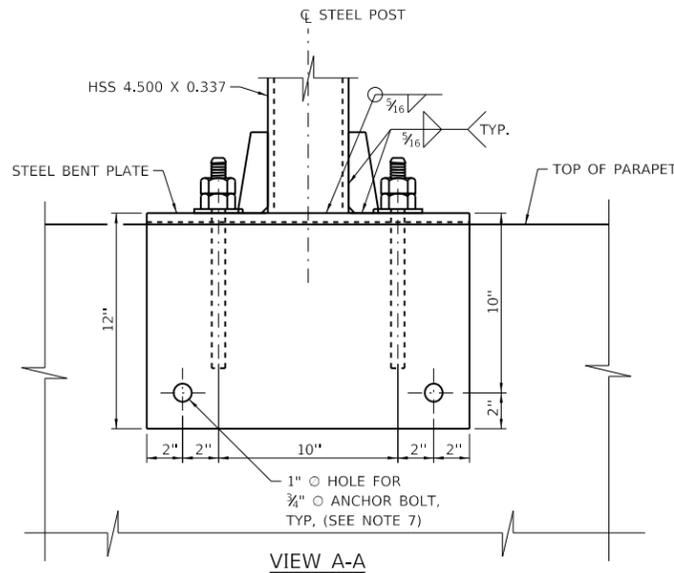
**POST INSTALLED DETAIL**
