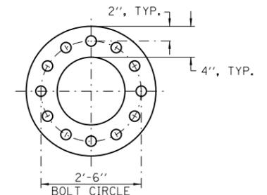
**POSITIONING PLATE/ANCHOR BOLT**
