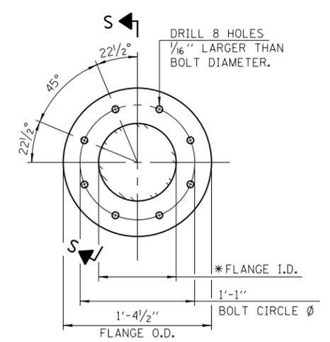
\*TO FIT O.D. OF CHORD WITH MAXIMUM GAP OF 1/16".
