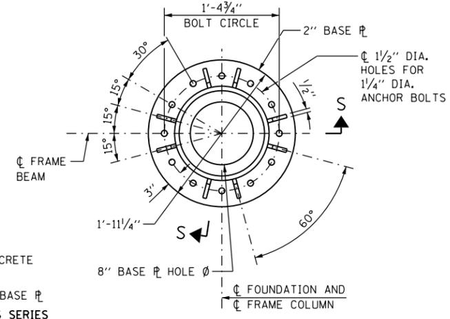
BASE PLATE PLAN MONOTUBE FRAME
