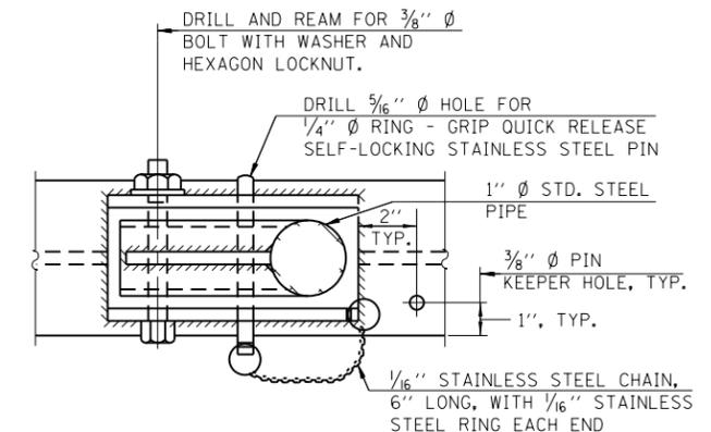
**PLAN AT HANDRAIL HINGE**
