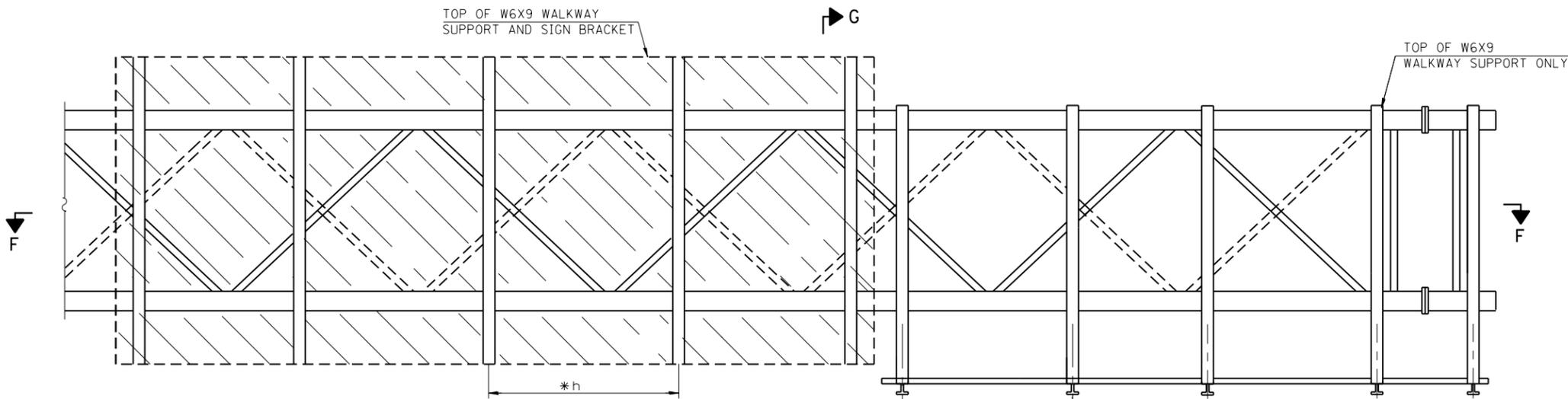
WALKWAY AND TRUSS GRATING WIDTH DIMENSIONS ARE NOMINAL AND MAY VARY  $\pm 1/2$ " BASED ON AVAILABLE STANDARD WIDTHS.
