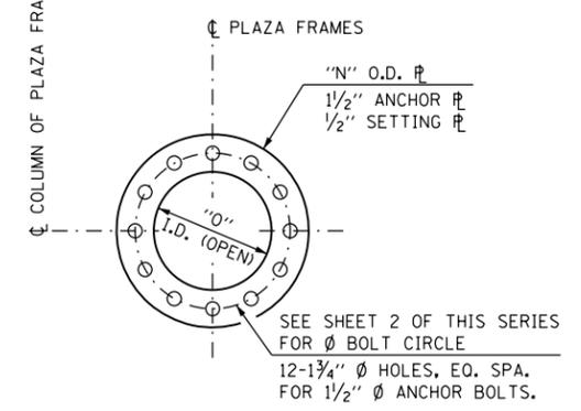
**ANCHOR PLATE / SETTING PLATE BAR LIST-ONE FOUNDATION**
