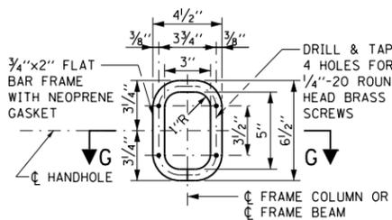
PROVIDE 6 1/2 inch x 4 1/2 inch #10 GA. COVER. ROUND CORNERS TO 1 3/4 inch RADIUS. PROVIDE FOUR 3/16 inch DIAMETER HOLES.
