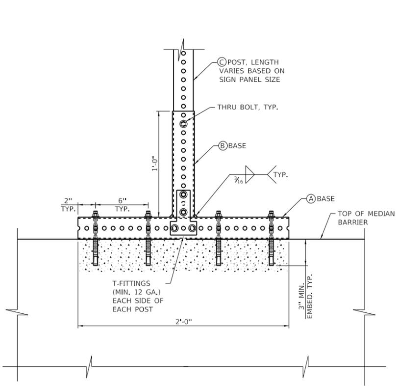
SIDE ELEVATION - BARRIER MOUNT DETAIL
