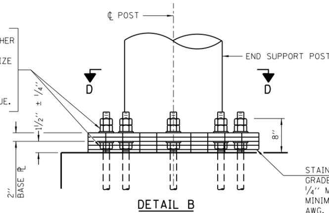
STAINLESS STEEL STANDARD GRADE WIRE CLOTH, 3" WIDE, 1/4" MAXIMUM OPENING WITH A MINIMUM WIRE DIAMETER OF AWG. NO. 16 WITH A MINIMUM 2" LAP. SECURE TO BASE PLATE AFTER ERECTION WITH 3/4" STAINLESS STEEL BANDING.
