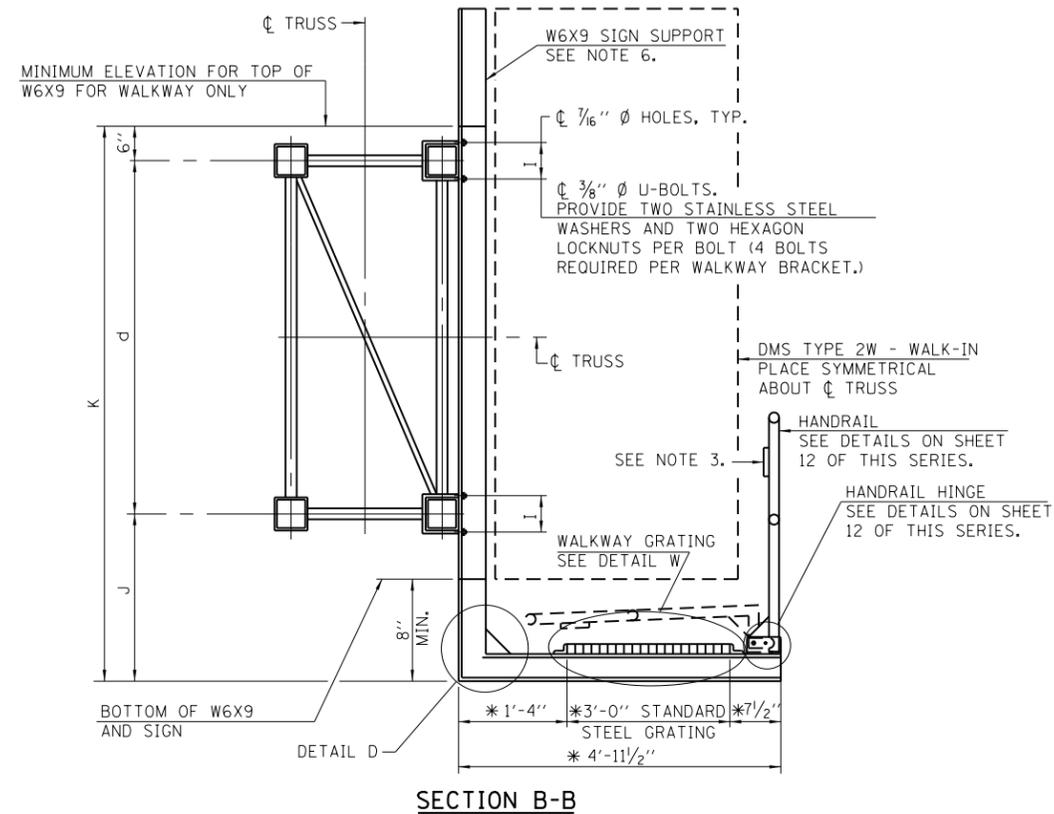
\*BRACKET AND GRATING DIMENSIONS ARE NOMINAL AND WILL VARY BASED ON ACTUAL DMS TYPE 2W - WALK-IN DIMENSIONS PLUS MANUFACTURERS MOUNTING DEVICE.
