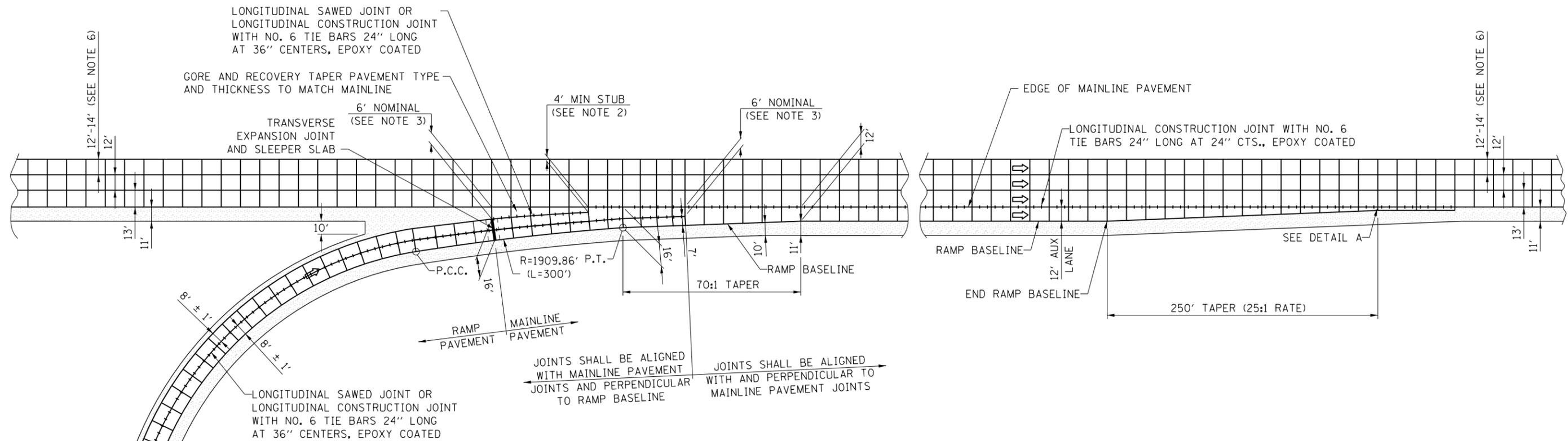
JOINTS SHALL BE ALIGNED WITH MAINLINE PAVEMENT JOINTS AND PERPENDICULAR TO RAMP BASELINE
