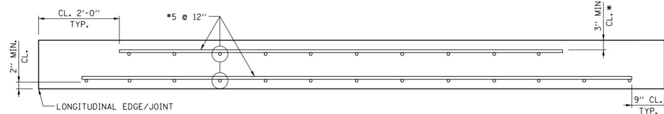
REINFORCEMENT SECTION A-A
