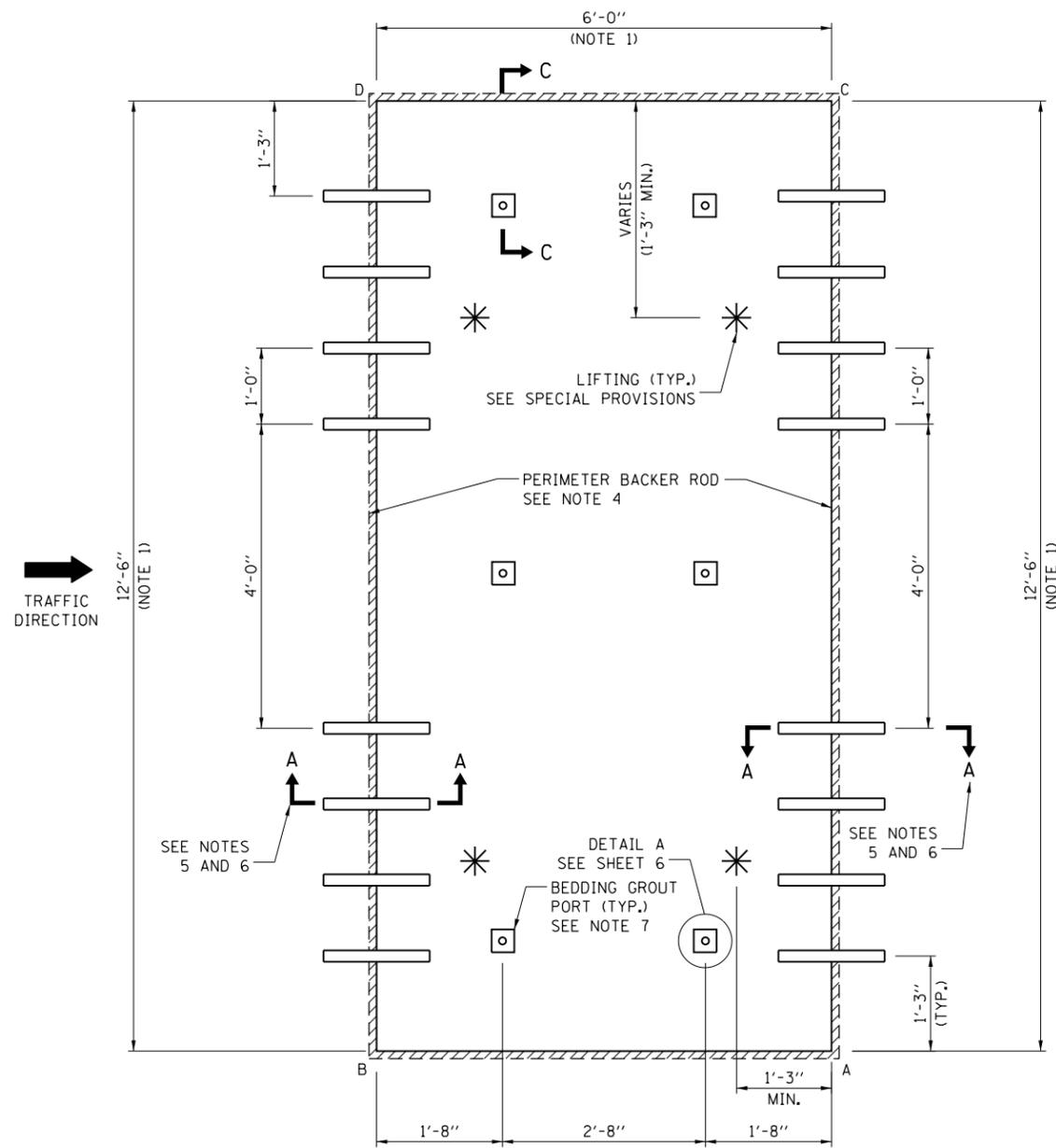
STANDARD 12'-6" WIDE PANEL LAYOUT FOR ISOLATED PLACEMENT
