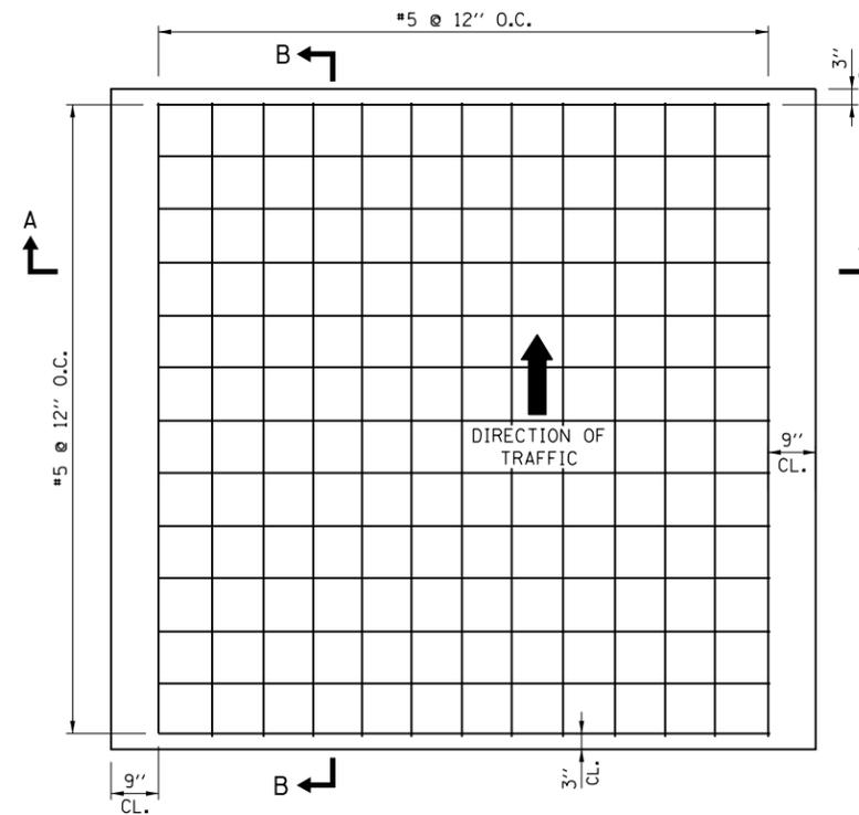
TYPICAL REINFORCEMENT DETAIL FOR STANDARD SLABS
