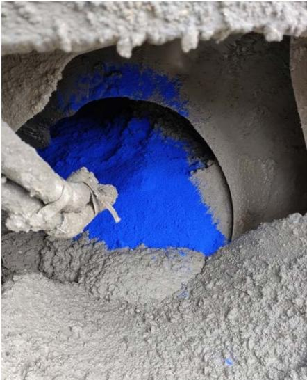
Figure 4-2. Addition of HydroMax
