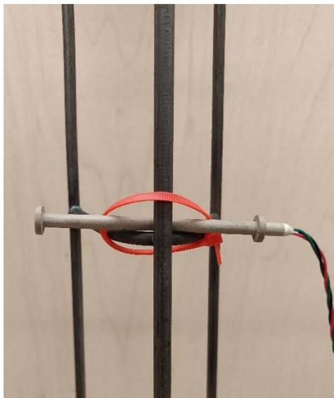
Figure 4-10. Strain gage secured to positioning chair with zip tie
