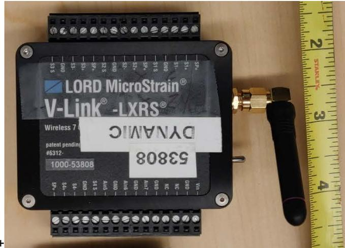
Figure 4-12. LORD MicroStrain V-Link wireless node
