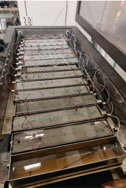
Figure 2-13. Test setup for frost durability
