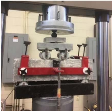
Figure 2-8. Test setup for flexural strength measurement of beam specimens
