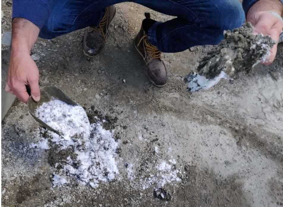
Figure 4-18. Dispersion issue seen during the BASF mixture pour
