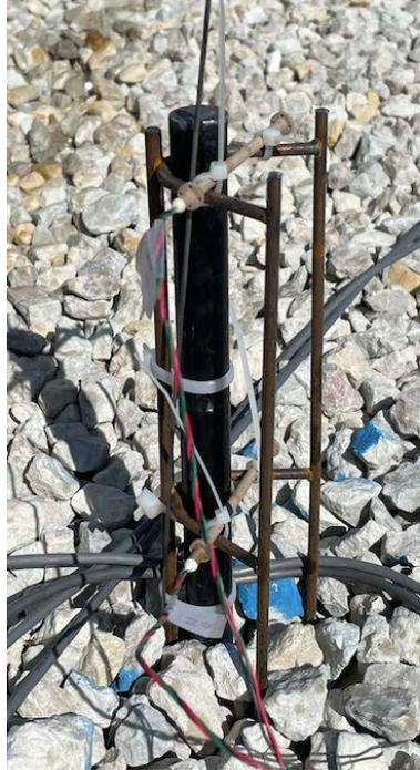
Figure 4-9. Strain gages mounted on positioning chair
