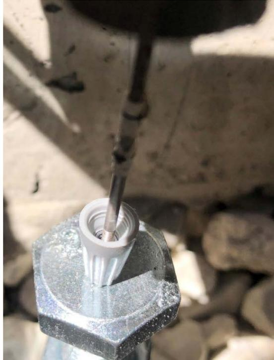
Figure 4-14. Connection between reference point and lift off gage (LVDT)
