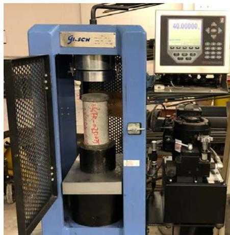
Figure 2-7. Test setup for compressive strength
