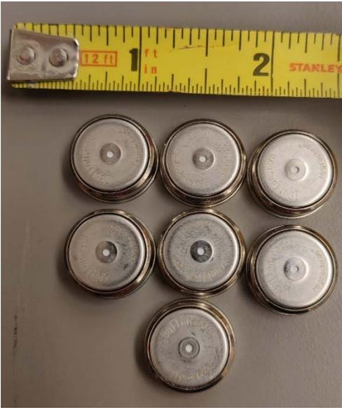
Figure 4-16. iButtons (temperature and relative humidity sensors)
