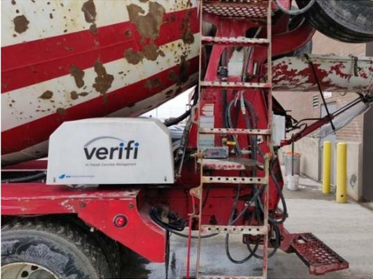
Figure 4-3. GCP applied technologies VERIFI® apparatus
