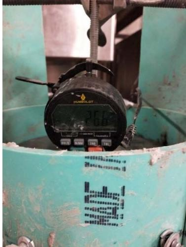
Figure 2-6. Surface settlement test
