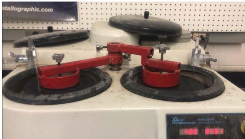
Figure 2-14. NANO 2000T grinder-polisher machine setup
